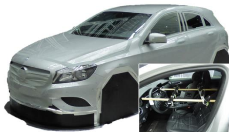
Figure 1: Mercedes-Benz A-class with blocked underbody flow and interior microphone array
