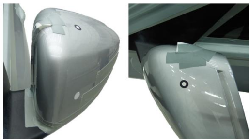
Figure 2: Side mirror modification (4 mm forward facing diffuser step)
