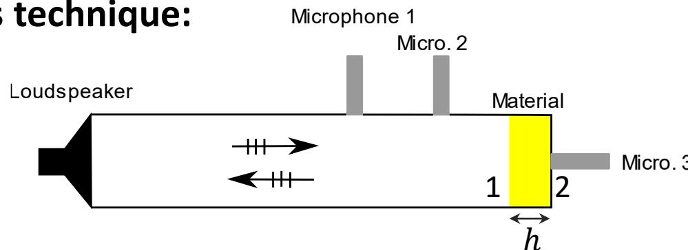
$$\begin{pmatrix} p_1 \\ v_1 \end{pmatrix} = [\mathbf{T}] \begin{pmatrix} p_2 \\ v_2 \end{pmatrix}$$
