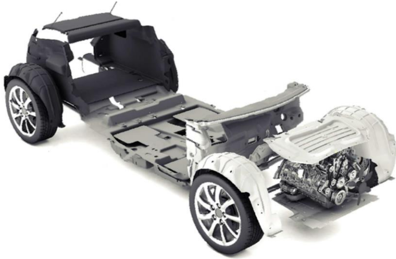
Figure 1. Use of porous materials to reduce the noise in the automotive industry. Source: Adler Pelzer.
